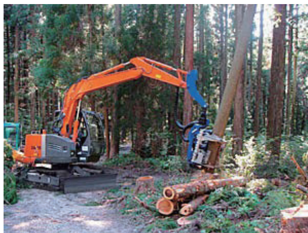
A self-propelled machine that performs felling, pruning, and accumulation of timber : a photo from the website of the Forestry Agency
